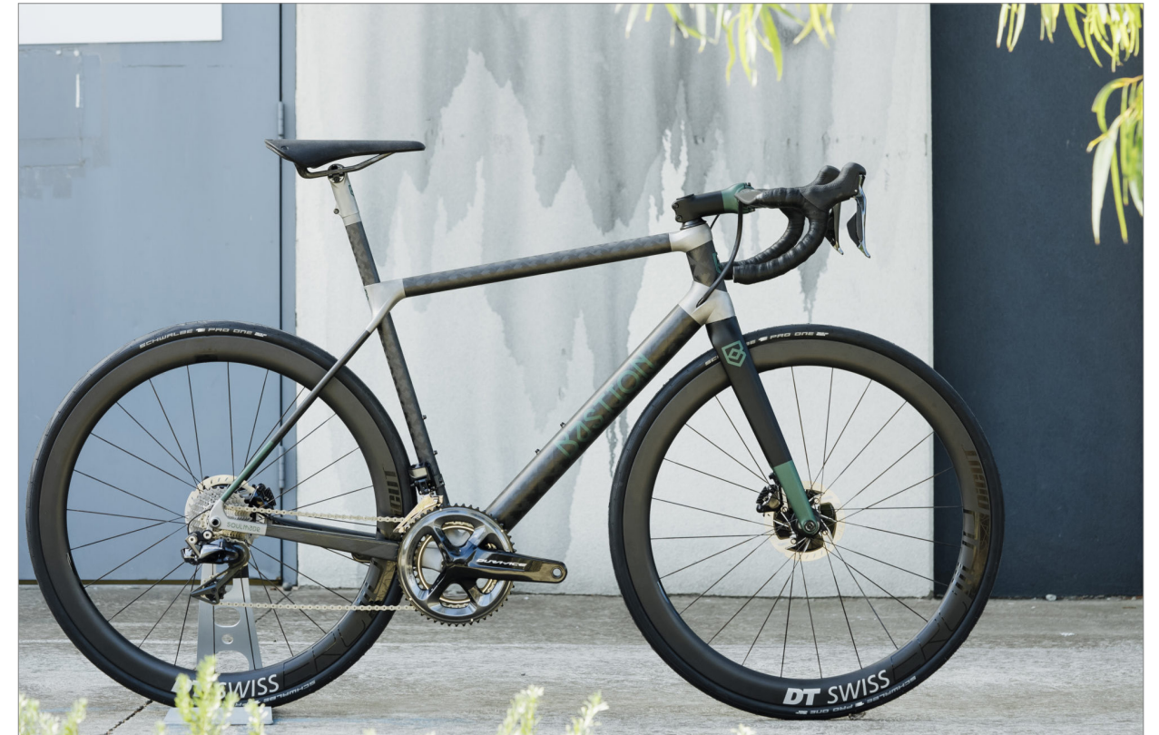
Fig. 8 This high-performance bicycle from Bastion Cycles made from carbon fibre tubing and AM titanium lugs. The resulting product is a very high strength, lightweight bicycle that is perfectly tailored to each individual customer
